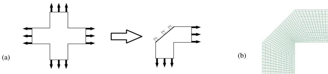
**Fig. 1:** Cross-shaped plate: (a) geometry; and (b) meshing.
