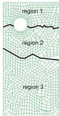
**Fig. 9:** Semi-structured regions of asymmetric cracked plate with a hole.
