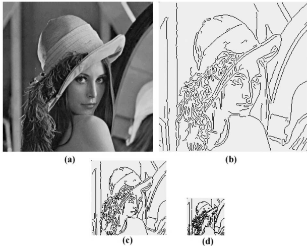
Fig. 2 Different levels of edge pyramid for a typical image (a) original image (b) edge image level 1 (c) edge image level 2 (d) edge image level 3.
