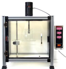
Fig. 1 Ultrasonic homogenizer (Sonicator) made in Iran by FAPAN Co. Ltd. with titanium probe and sound absorbing box.
