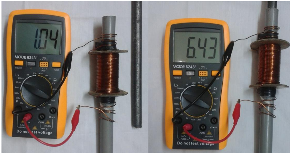
Figure 4. increasing coil inductance using a rotar longer than the coil
