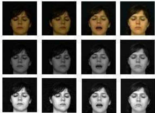
Fig. 2. The result of histogram equalization. Original images (top row), grayscale images (middle row) and images after histogram equalization (bottom row).
