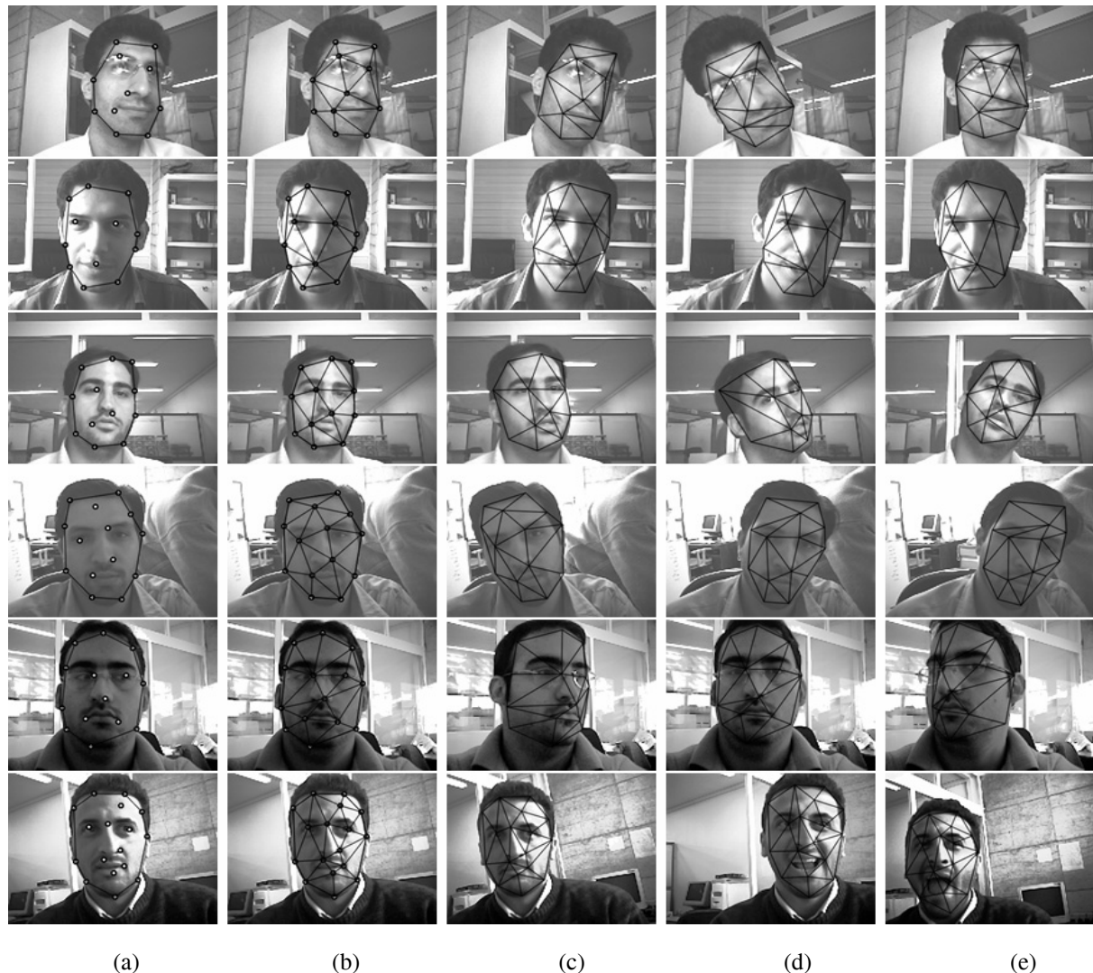
Fig. 8. Results of the proposed face tracking algorithm for six different videos (A, B, C, D, E, and F); (a) face features and contour extraction (b) face mesh generation (c) ,(d) ,(e) results of the tracking algorithm at different video frames; the first row: frames 70, 149, and 200; the second row: frames 40, 85, and 190; the third row: frames 112, 132, and 198; the fourth row: frames 45, 145, and 192; the fifth row: frames 90, 128, and 158; the sixth row: frames 58, 149, and 239.
