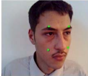
Figure 1. Four markers on the face for camera mouse implementation
