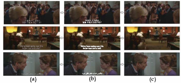
Fig. 8: The results of text localization and inpainting algorithm (a) original images, (b) the extracted texts, (c) the reconstructed images after applying the proposed text extraction and inpainting algorithm.
